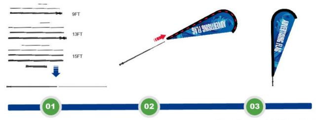
Align the pole structures from smallest to largest before assembly. 3 types of poles available
